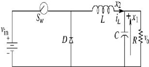
Fig. 2. Dc-dc buck converter topology.
