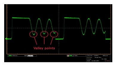
Fig. 6. Quasi-resonant switching waveform for a fly back converter (Courtesy of Infineon Technologies).
