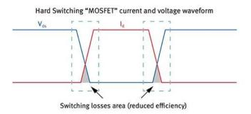
**Fig. 4.** Voltage regulator losses occur during voltage/current overlap when the MOSFET switches (Courtesy of Infineon Technologies).
