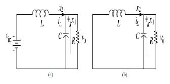
Fig. 3. Buck converter circuit when switch: (a) turns on (b) turns. Off.
