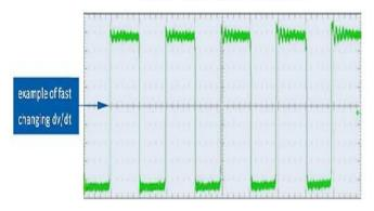
**Fig. 5.** Manufacturers increase dv/dt to minimize overlap and improve efficiency (Courtesy of Infineon Technologies).
